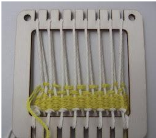
Weft is being pulled too tight.
